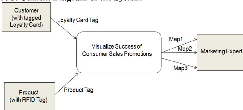
DFD 0 shows the subprocesses of the system, their interaction with each other and with the environment of the system.
