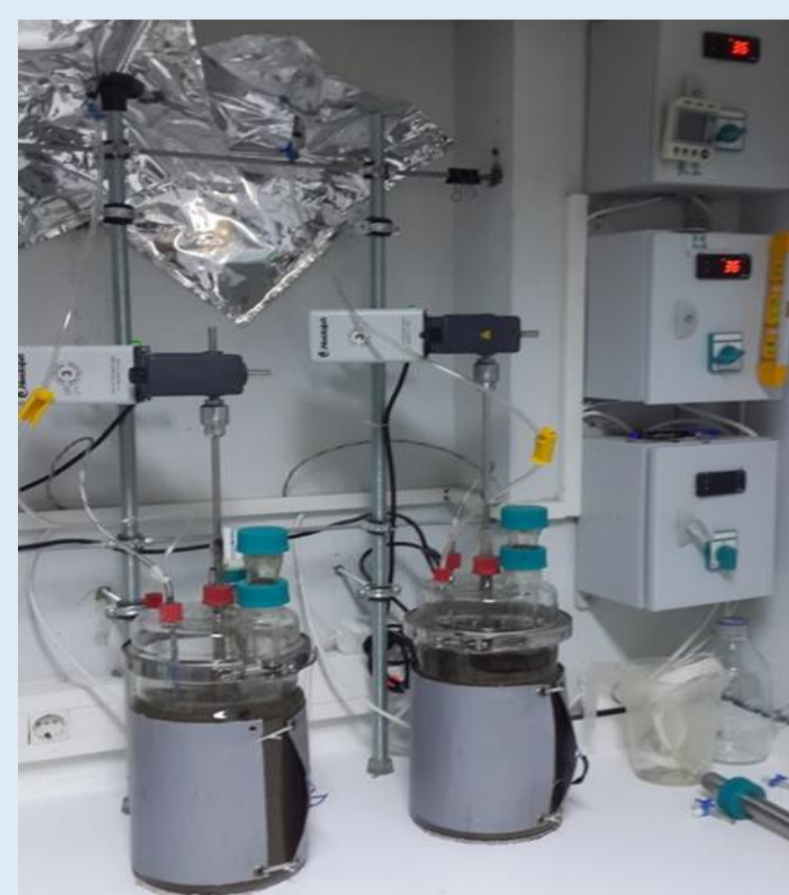
Figure [1]: Photograph of CSTR-C and CSTR-M operated under the same conditions
