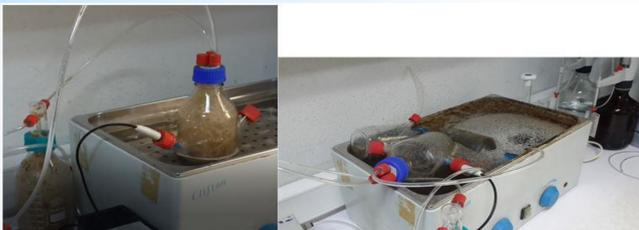
Figure : Foaming problem in ammonia stripping process that includes ventilation with diffuser.
