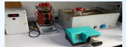
Figure : The photograph of the setup used in batch experiment with using tubular PP membrane
