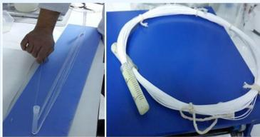
Figure : Preparation of the hydrophobic hollow fiber membrane (HFM) module
